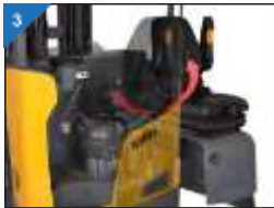
One-piece cover The cover can be opened to ensure the maintenance easy and fast.
