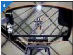
Wide view mast The mast system and roof guard adopt new structure, optimize operators' view.
